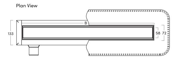
STRUCTURAL LENGTH - A VISUAL LENGTH - B DRAIN DEPTH - C 660mm 600mm 99mm
