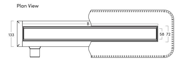
STRUCTURAL LENGTH - A VISUAL LENGTH - B DRAIN DEPTH - C 960mm 900mm 99mm
