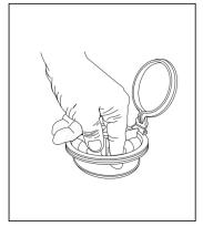
Remove the grate. Pull trap out of the drain and clean. Place back into the drain.
