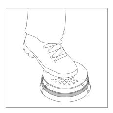
Push the clamping ring and grate down into the drain.
